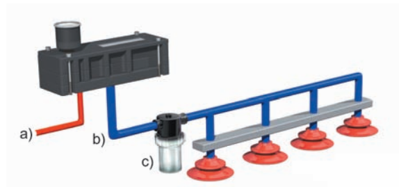
1. Centralized system. a) Compressed air, b) Vacuum, c) Vacuum filter
